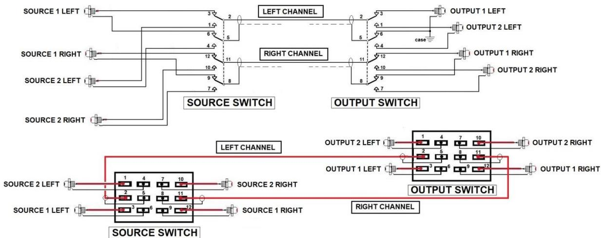
**SOURCE SWITCH** - The Left and Right circuits are identical apart from the switch sections used.
